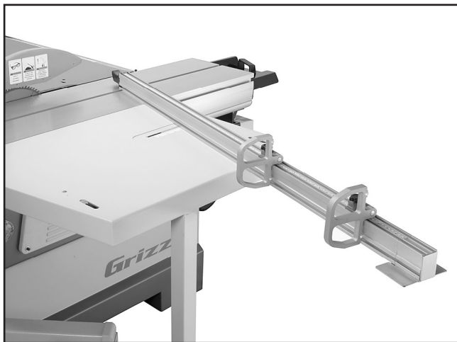
Figure 62. Fence set-up for angled cuts.
